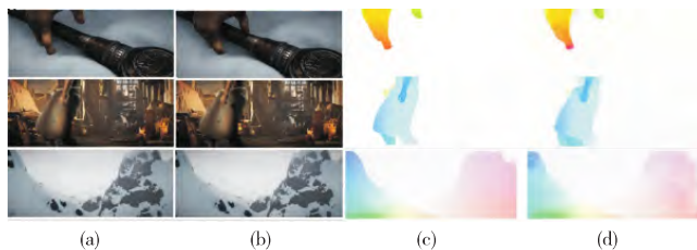
图1 DS-PWC 在 Sintel 训练集上的结果及与真实光流的对比 Fig. 1 DS-PWC results on the Sintel training set and comparison with real optical flow
