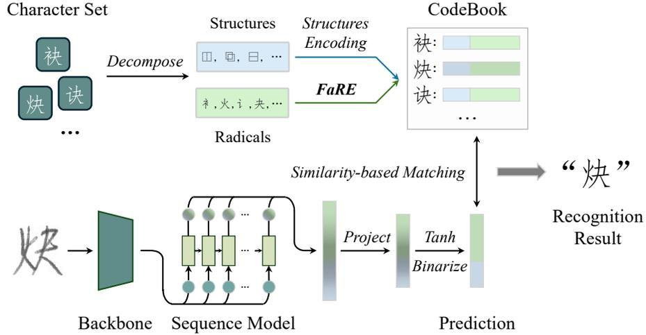
Fig. 4: The overall architecture for character recognition using FaRE.
